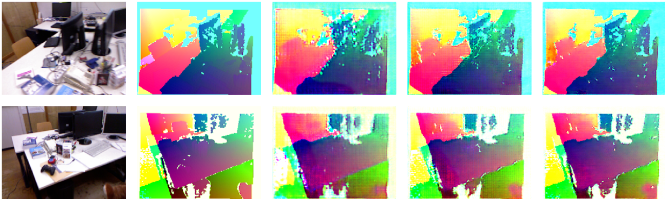
Fig. 1. The generative network learns to map from RGB images to 3D coordinates that can be processed through geometric algorithms to recover the camera pose even after extreme occlusion. From left to right, the RGB frame, the Cartesian scene coordinates ground truth, and GAN outputs after 10, 30, and 70 epochs of training.
