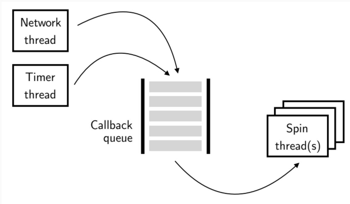
**Figure 1:** Network and spin threads interact through the callback queue
